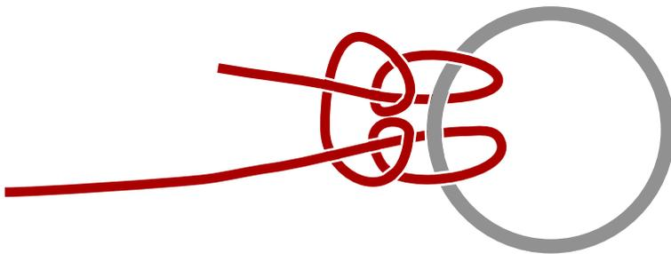
Pass loop down over ring and lines, and draw loop tight by pulling on both legs of line and the ring.
